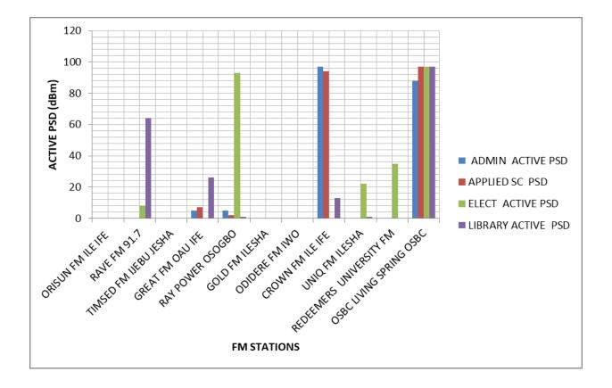
Figure 4: FM Stations Active Power Spectral Density Distribution within 8 hours period.
