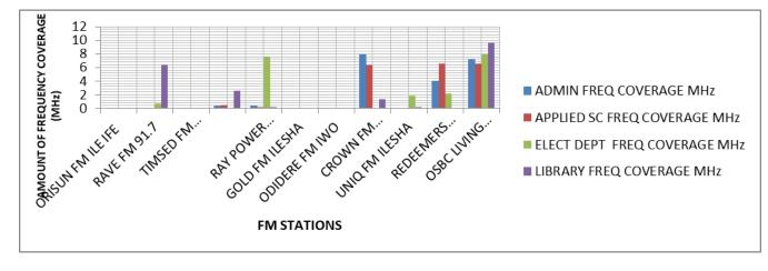
Figure 7: FM Stations Spectrum Utilization Profile within 8 hours period
